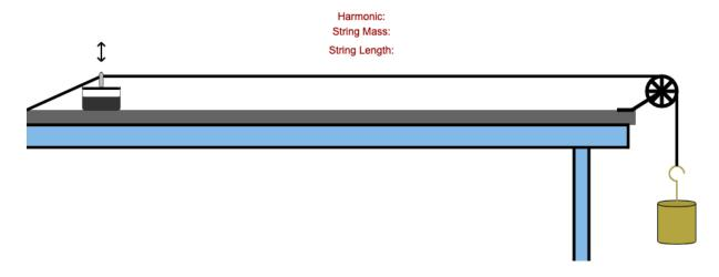
Step 2: Calculate the force tension from the hanging mass
