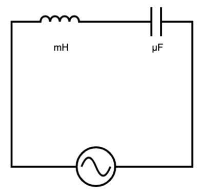
Step 2: Neatly calculate the impedance of the capacitor and the impedance of the inductor for this frequency.
