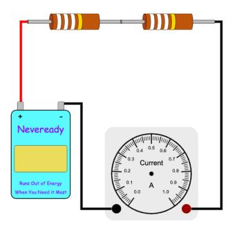
Step 2: Find the resistance of your resistor based on the color code and then find the total resistance of the combination of resistors. Show how you did this in the space below
